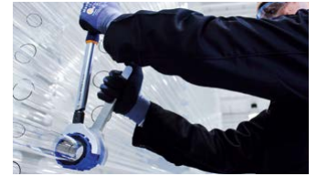
8 Now turn the wrenches in opposing directions until the torque wrench tilts towards your body. The connection process is now completed.
