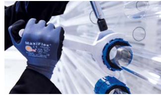
7 The jaw wrench should be placed accordingly on the right side of the coupling.
