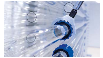
6 Take the correct torque wrench and place it on the left side of the coupling. Required torque for Standard Couplings is 40 Nm, for Slim Couplings it is 25 Nm. It is important to affix the draw-hook of the tool on the side averted to the body. Make sure there is enough space for the torque wrench to tighten.
