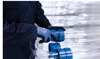
9 Repeat these steps with all other couplings. For the connection of the tube levels please use the U-Bends. The installation of the couplings at the U-Bends is the same as shown before. First, affix two couplings to the U-Bend up to the spacers inside the cages.
