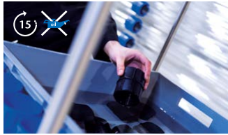
2 Place the cages into warm water (approx. 50°C / 122°F) for a minimum of 15 minutes to allow an easier gliding of the cage over the tube end. The water will lubricate and expand the cage. Please do not use any other lubricants, such as oils or silicones.
