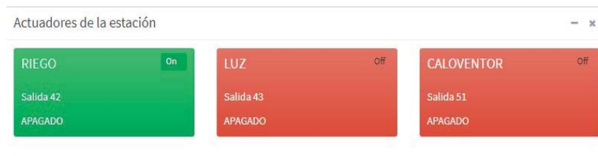
Fig. 9. Actuator control from the webpage
