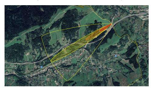
**Figure 7.** Graphical representation of the dispersion of a dangerous substance at the Skalité-Zwardoň-Myto 2 border crossing [24,25].
