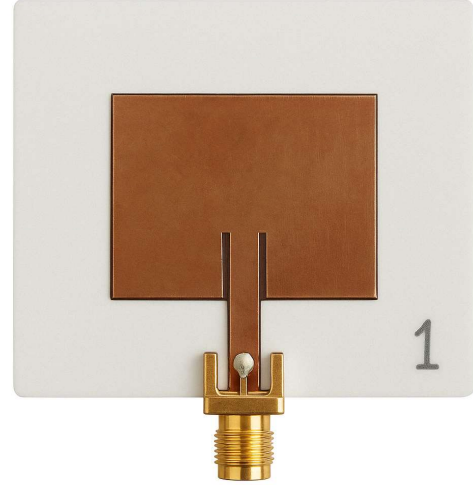
First geometry Patch Antenna
