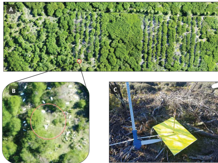
Fig. 4. Collocation marks: (A) general view of the orthomosaic, (B) amplified view of the orthomosaic showing one of the marks, and (C) fixed plot center mark used during the field sampling. [Color online.]
