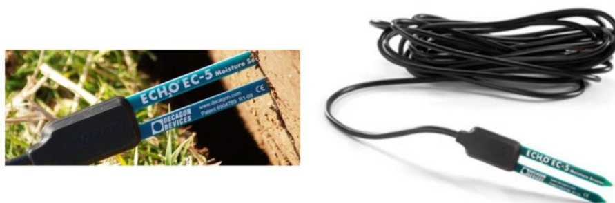
Figura 15: Sensores ECH 2 O EC-5 Decagon® tomado de: http://www.decagon.com/
